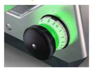
Green means motor off gauge plate closed.
